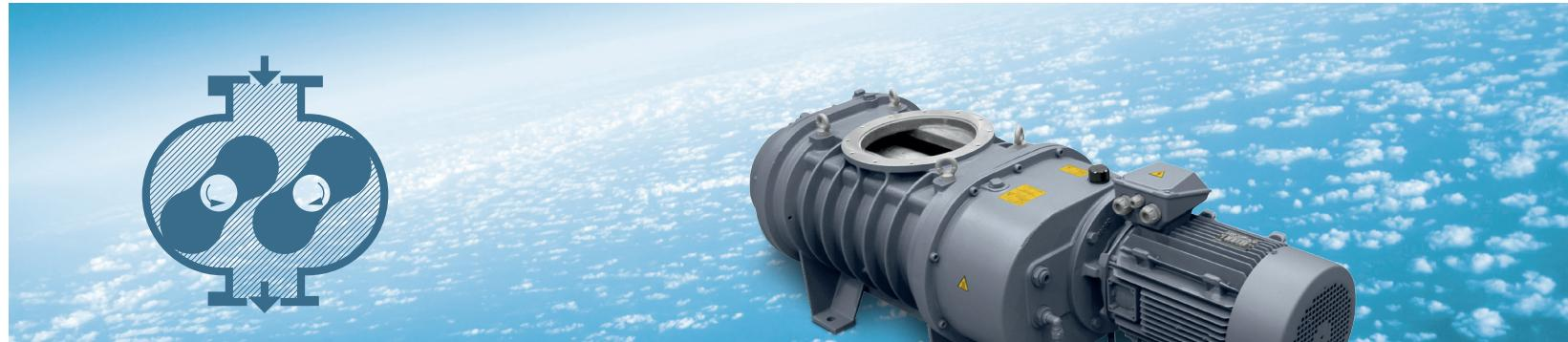
The ZRS mechanical booster pumps, based on the simple roots principle, remains the favourite pump for applications where high pumping speeds are required for pressures in the region of 0.01 to 10 mbar. This pump must always be backed by another pump, which can deliver against a high-pressure differential to
